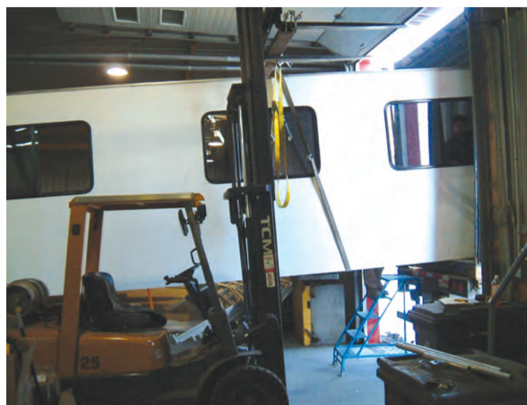
The houseboat's huge pontoons (top) and clinic walls are loaded into a shipping container, to be reassembled later in Gabon.
